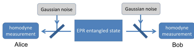
Fig. 4. Schematic of transmitting an EPR entangled state in two Gaussian thermal noise channels.
