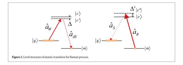
entanglement enhancement can be achieved. By applying another strong read field  $\hat{a}_R$ , the entanglement between atomic ensemble and anti-Stokes field is converted into entanglement between Stokes and anti-Stokes fields, which is used for verifying atom-light entanglement.
