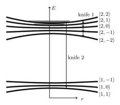
**Fig. 2.** Microwave and Radio frequency induced transitions for evaporating the <sup>87</sup>Rb cloud in  $F=2, m_F=2\rangle$  state. The knife 1 indicates Radio frequency induced transitions, and the knife 2 shows microwave induced transitions.
