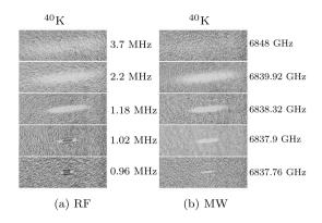
**Fig. 3.** False colour absorption images of <sup>40</sup>K in QUIC trap at four different stages of the sympathetic cooling. Panel (a) shows the <sup>40</sup>K atoms in the RF induced evaporative cooling stage, and panel (b) displays the <sup>40</sup>K atoms in the MW induced evaporative cooling stage.
