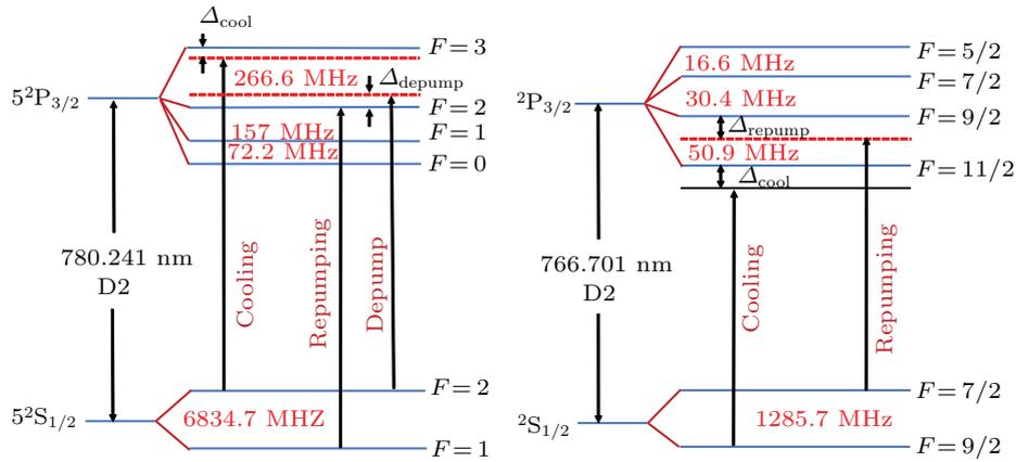
**Fig. 2.** Hyperfine structure of D2-line of  $^{87}\text{Rb}$  and  $^{40}\text{K}$ . (a) Transitions of  $^{87}\text{Rb}$  D2 line for the cooling light, repump light and depump light. (b) Transitions of  $^{40}\text{K}$  D2 line for the cooling and repump light.
