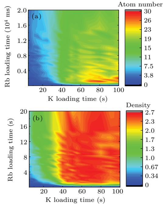
**Fig. 6.** The optimization of rubidium and potassium loading time. (a)  $^{40}\text{K}$  atom numbers and (b) optical density as the function of rubidium and potassium loading time by dark MOT loading. Horizontal axis represents for the Rb loading time, vertical axis represents for the  $^{40}\text{K}$  loading time, and color gradient represents the number and density of  $^{40}\text{K}$  atoms, respectively.
