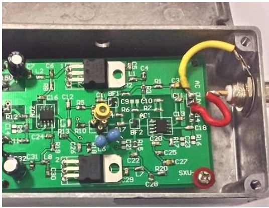
Fig. 3. Photograph of the amplifier. Many components are surface mounted (packaged in 0805), and the output connectors are all 50 Ω-BNCs.
