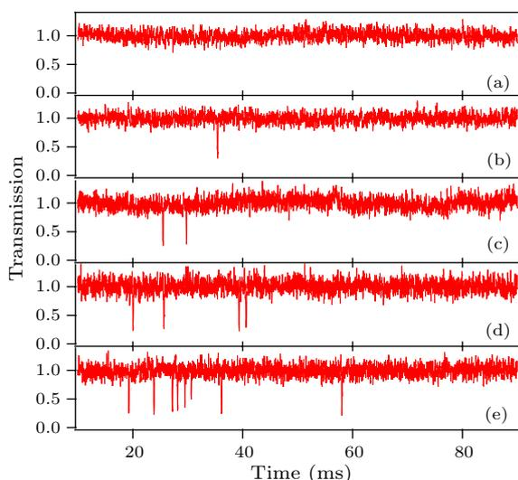
**Fig. 3.** The time-varying cavity transmissions with repetitive drops. There are 0, 1, 2, 4 and 8 atoms [(a)–(e)] flying through the cavity mode, respectively.
