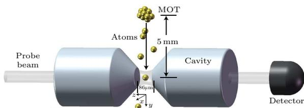
**Fig. 1.** (Color online) Schematic of the experimental setup. The length of the cavity is  $86 \mu\text{m}$ . The finesse of cavity is  $F = 330000$  and the parameters of the system are  $(g_0, \kappa, \gamma) = 2\pi \times (23.9, 2.6, 2.6)$  MHz. The MOT with about  $10^5$  atoms is positioned at  $5 \text{ mm}$  above the cavity. The atoms fall down and through the cavity mode after shutting off the MOT and the transmissions of the cavity are detected by the SPCMs.
