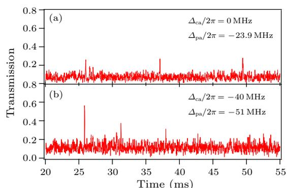
**Fig. 5.** The cavity transmission spectra with different probes and cavity detunings when the atom passes through the cavity mode. (a)  $\Delta_{ca}/2\pi = 0$  and  $\Delta_{pa}/2\pi = -23.9 \text{ MHz} = -g_0$ , (b)  $\Delta_{ca}/2\pi = -40 \text{ MHz}$  and  $\Delta_{pa}/2\pi = -51 \text{ MHz}$ .
