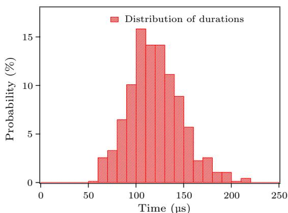
**Fig. 4.** Histogram of atom durations inside the cavity. The duration is obtained by the full width half maximum of the dips. The average atom duration is about  $110 \mu\text{s}$ .
