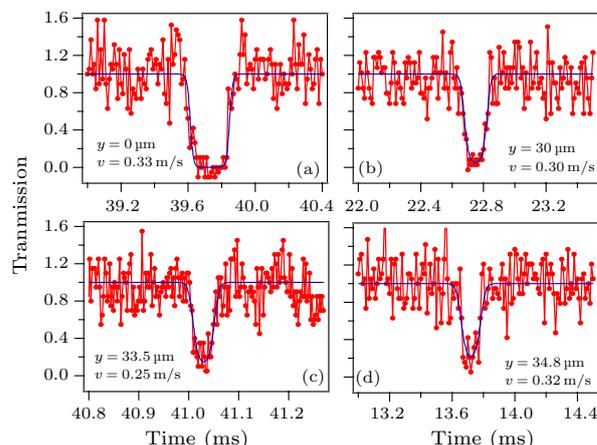
**Fig. 2.** The cavity transmissions versus time with atoms passing through the TEM<sub>00</sub> mode of cavity for  $\Delta_{ca} = \Delta_{pa} = 0$ . The intra-cavity mean photon number is  $m \approx 1$ . The atom is released at  $t=0$  with shutting off the MOT. The position and the velocity of the atom for each transit are shown.
