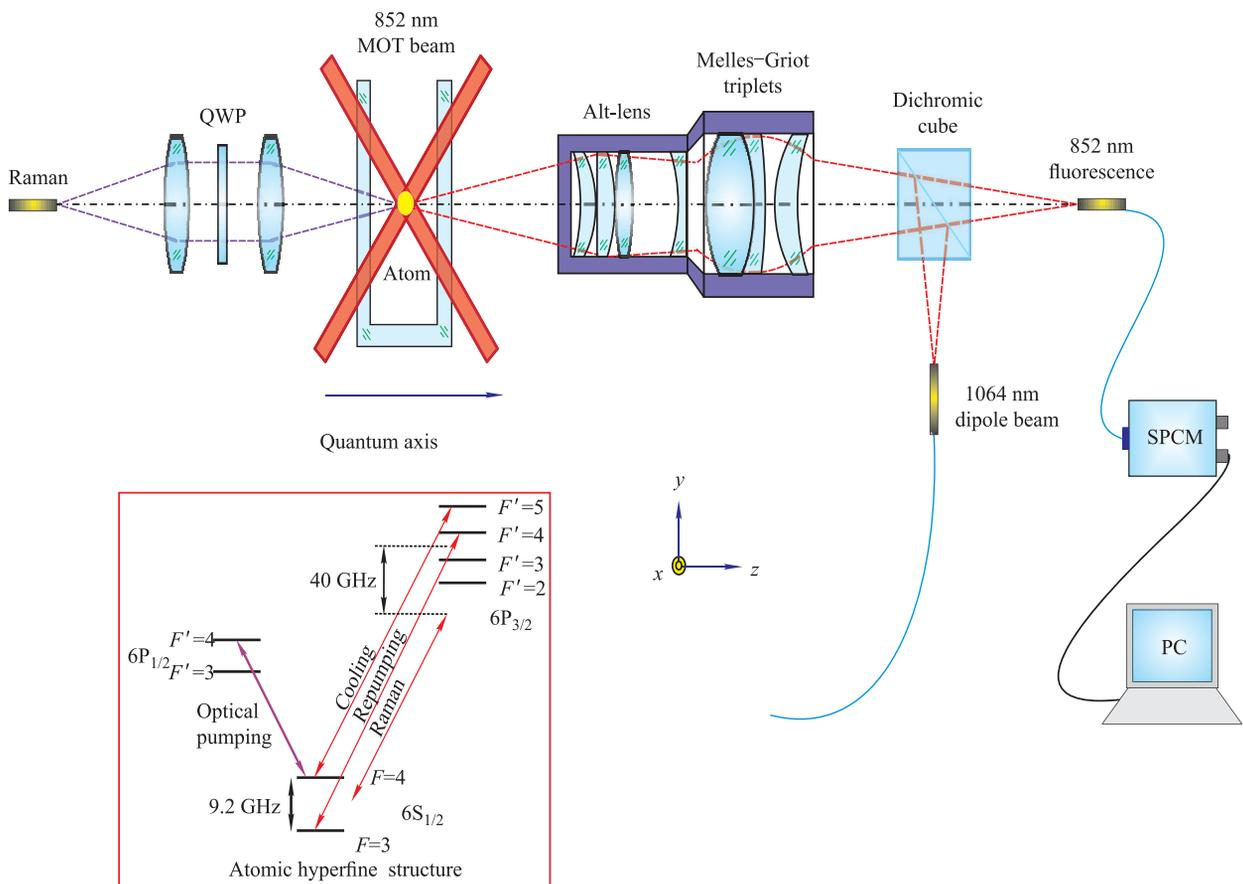
**Fig. 1** The experimental setup. A tightly focused beam (FORT beam) by Alt-lens overlaps exactly with the MOT. Fluorescence light scattered by the trapped atom is collected by the same objective and separated from the FORT beam by a dichromic cube. The quantization axis is defined by a 2 Gauss magnetic field along the  $z$  axis. The inset shows the relevant atomic hyperfine structure of  $^{133}\text{Cs}$  and the corresponding driving beam used to manipulate the single-atom qubit.
