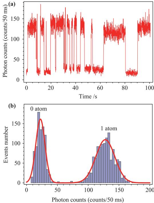
**Fig. 2** Typical signal from single atoms. (a) Fluorescence recorded by the single counter and (b) the corresponding histogram.
