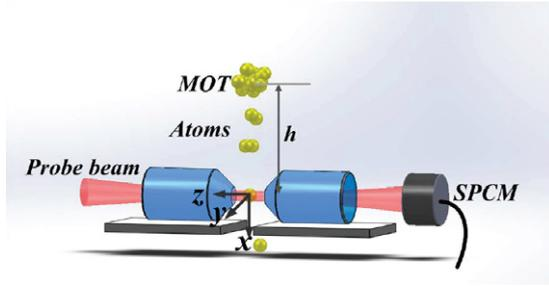
**Figure 1.** Schematic of our experimental setup. The microcavity consists of two super-mirrors. The cold atom cloud is produced in a MOT right above the centre of the cavity. The SPCM is used to detect the cavity output. Atoms fall freely from the MOT under gravity and pass through the cavity mode.
