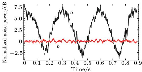
**Fig. 4.** (color online) Plots of squeezing at 35 kHz versus time, where (curve *a*) black line represents the normalized quantum noise power of the squeezed vacuum at the Cs D2 line when the LO phase is scanning, while (curve *b*) red line refers to the normalized SQL with RBW = 1 kHz and VBW = 300 Hz.
