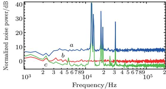
**Fig. 3.** (color online) Measured noise spectra for (curve *a*) anti-squeezed light, (curve *b*) the SQL, (curve *c*) squeezed light after correction of the electronic noise (15 dB below the SQL) of the HD system. RBW = 100 Hz, VBW = 10 Hz. Sweep time = 19.6 s. All traces are averaged over 10 times.
