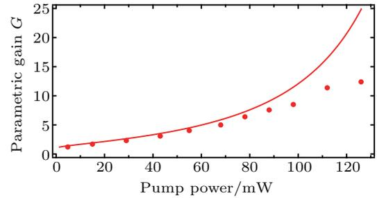
**Fig. 2.** (color online) Parametric gain versus pump power, where solid line represents the theoretical simulation results and solid circles denote experimental results.
