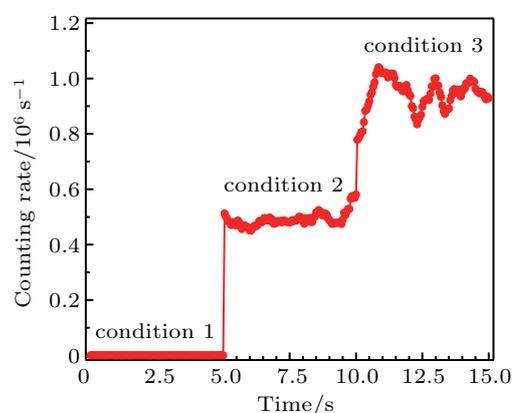
**Fig. 2.** Counting rate of the SPCM from atomic fluorescence collected by the nanofiber versus time for three experimental conditions. In condition 1, all the MOT beams and magnetic field are switched off. In condition 2, all the MOT beams are switched on and the magnetic field is still switched off. In condition 3, all the MOT beams and the magnetic field are switched on.
