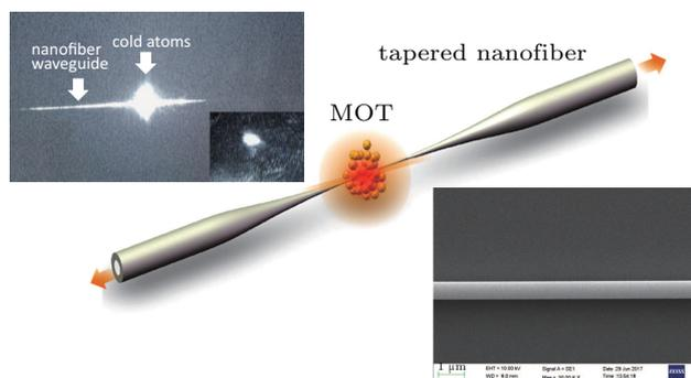
**Fig. 1.** Schematic diagram of the experimental setup: the nanofiber overlaps with the cold atom cloud. The upper-left figure shows the CCD image of cold atoms and the nanofiber. The lower-right figure shows a typical SEM image of a nanofiber.
