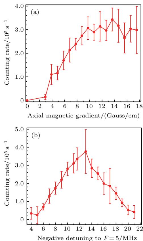
**Fig. 4.** (a) Counting rate from the fluorescence of cold atoms as a function of axial magnetic gradient. The detuning of cooling beams is  $-11.6 \text{ MHz}$ . (b) Counting rate from the fluorescence of cold atoms as a function of detuning. The axial magnetic gradient is  $11.7 \text{ Gauss/cm}$ . The intensities of cooling and re-pumping beams are  $33.6 \text{ mW/cm}^2$  and  $35.4 \text{ mW/cm}^2$  for both figures.
