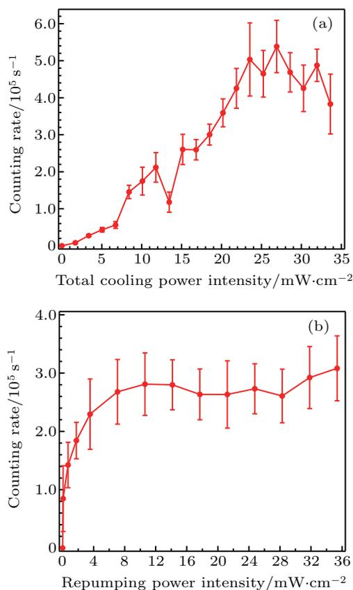
**Fig. 3.** (a) Counting rate from the fluorescence of cold atoms as a function of the intensity of the cooling beams. The intensity of the re-pumping beam is  $35.4 \text{ mW/cm}^2$ . (b) Counting rate from the fluorescence of cold atoms as a function of the intensity of the re-pumping beams. The intensity of the cooling beam is  $33.6 \text{ mW/cm}^2$ . The detuning of the cooling beam is  $-11.6 \text{ MHz}$  and the axial magnetic gradient is  $11.7 \text{ Gauss/cm}$  for both cases.
