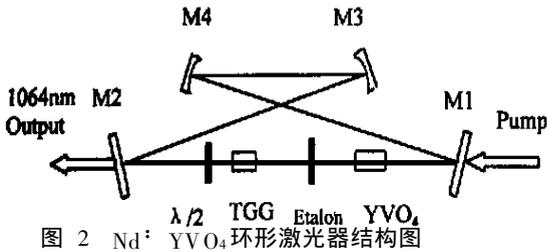
图 2 Nd:YVO<sub>4</sub> 环形激光器结构图Fig. 2 Configuration of Nd:YVO<sub>4</sub> ring laser
