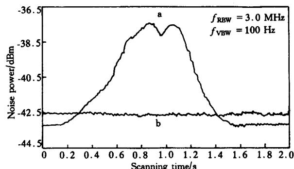
Fig. 7 The FM spectrum of saturated cesium vapor cell with squeezed light at analysis frequency of 15 MHz. a: the FM spectrum of  $D_2$  line of Cs atoms with Doppler broadening ( $6^2S_{1/2}F=4 \leftrightarrow 6^2P_{3/2}F'=3,4,5$ ); b: the shot noise limit
