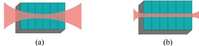
**Fig. 2** (a) Periodically-poled bulk crystal: the Gaussian laser beam is focused into the crystal with a focus waist. (b) Periodically-poled waveguide: the laser beam is coupled into the waveguide and confined in it. The accepted laser power is usually less than 250 mW to avoid damaging the waveguide structure.
