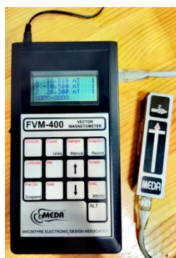
Fig. 3 Model FVM-400 three-axis fluxgate magnetometer from MEDA, USA. Left hand, the instrument panel; Right hand, the three-axis fluxgate detector head.
