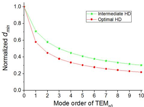
FIG. 1. Mode-order dependence of minimum measurable displacements for intermediate homodyne detection and optimal homodyne detection.
