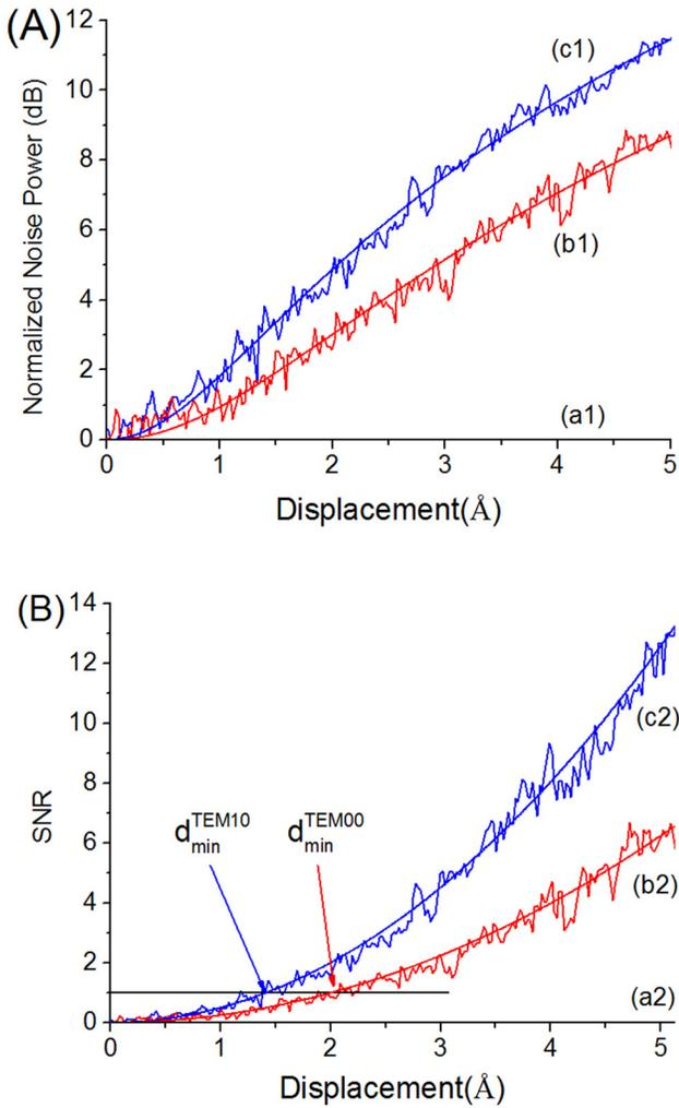
FIG. 3. (a) Normalized signal power measured in the ESA vs beam displacement: (a1) corresponds to the quantum noise, (b1)  $TEM_{00}$  signal mode, and (c1)  $TEM_{10}$  signal mode. (b) Signal-to-noise ratio plotted against displacement. Traces (a2), (b2), and (c2) correspond to traces (a1), (b1), and (c1), respectively.
