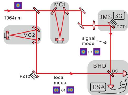
FIG. 2. Experimental setup. MC1, MC2: mode converters, DMS: displacement modulation system, PZT1, PZT2: piezoelectric transducers, SG: signal generator, BS: 50/50 beam splitter, BHD: balanced homodyne detection, ESA: electronic spectrum analyzer.
