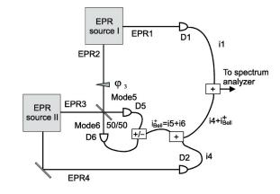
FIG. 3. Entanglement swapping, direct analysis of the photocurrents.
