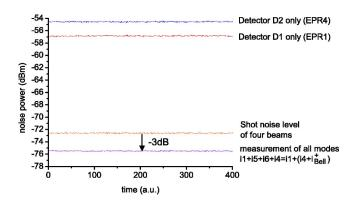
FIG. 7. Four-partite correlations: The measurement of all four modes gives a signal that is 3 dB below the corresponding shotnoise level. Thus, the generated four-mode state is highly correlated, each individual beam having a high noise level. The measurement time was 10 s. The measured noise traces are not corrected for the electronic noise which was at -87.8 dBm.
