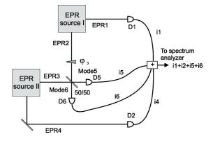
FIG. 6. Generation of a highly correlated four-partite state.
