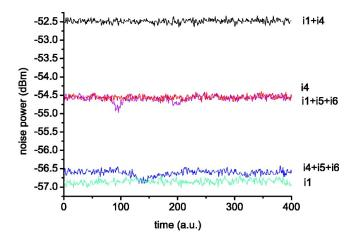
FIG. 8. Correlations of the four-mode state. Measurement of three modes compared with the noise levels of the indivdual beams. The measurement time was 10 s. The shot-noise level for three modes is about -73.7 dBm.
