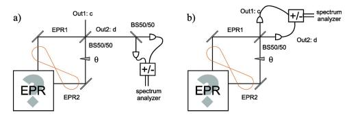
FIG. 9. Two possible setups for an indirect measurement of correlations in the phase quadrature of two beams EPR1 and EPR2. Both input beams are superimposed on a 50:50 beam splitter. In (a) the noise variance of one output port is detected. This also provides a direct measure for the nonseparability of states EPR1 and EPR2. In (b) the signal from both output ports is detected and the difference channel provides information about the correlations of the phase quadrature of beams EPR1 and EPR2.
