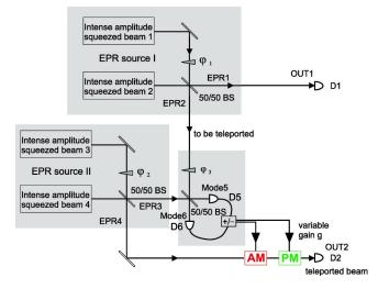
FIG. 1. Schematic drawing of the entanglement swapping experiment.
