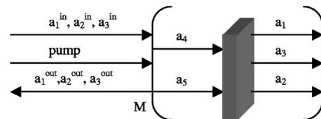
FIG. 1. Sketch of the OPO.  $a_4, a_5$  are pump beams. Pump  $a_4$  creates fields  $a_1$  and  $a_3$  by the process of parametric down conversion, and simultaneously pump  $a_5$  and field  $a_3$  produce sum-frequency field  $a_2$ .  $a_j^{\text{in}}$  ( $j=1,2,3$ ) are the incoming fields.  $a_j^{\text{out}}$  are the corresponding outgoing fields.
