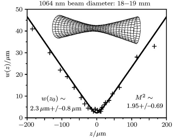
**Fig.2.** Measurement of the extremely small waist of the 1064 nm laser beam (with a beam diameter of 18~19 mm), which is strongly focused by a lens assembly. The radius of the waist is  $2.3 \pm 0.8 \mu\text{m}$  with an  $M^2$  factor of 1.95.
