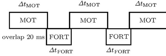
**Fig.3.** Time sequence of single atoms transferring between the MOT and the FORT with an overlap time of 20 ms. The storage time of a single atom in the FORT is  $\Delta t_{\text{FORT}}$ .
