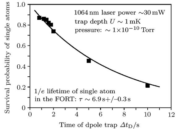
**Fig.5.** Survival probability of one single atom transferring between the FORT and the MOT as a function of time without cooling light. The fitting of the experimental data with exponential decay yields a  $1/e$ -fold lifetime of  $6.9 \pm 0.3$  s (1 Torr=133 Pa).
