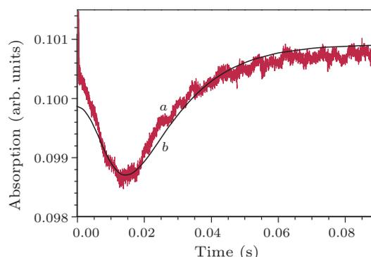
**Fig. 7.** Measured TOF signal (*a*) and the simulative calculation (*b*) in the compressed MOT, corresponding to temperature of about  $300 \mu\text{K}$ .
