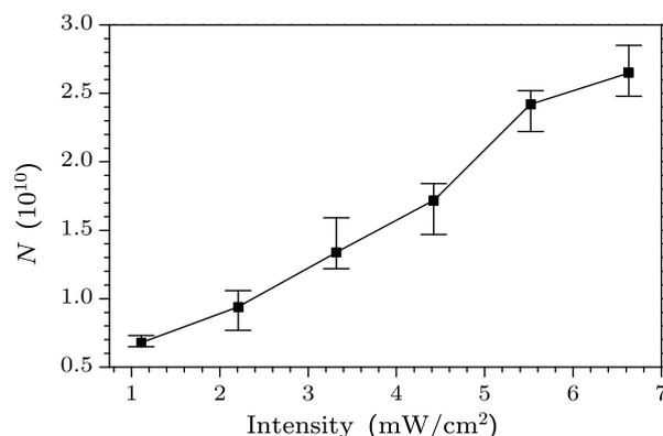
**Fig. 2.** Measured the number of the cold atoms as a function of the intensity per cooling laser.
