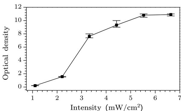
**Fig. 4.** Measured on-resonance optical density  $D(0)$  as a function of intensity per cooling laser.
