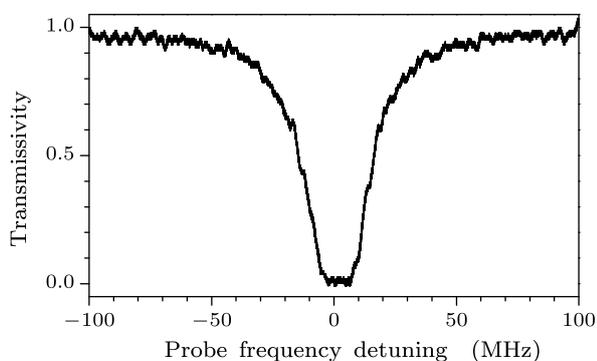
**Fig. 3.** Absorption spectrum of trapped Rb atoms, corresponding to optical density of 11.
