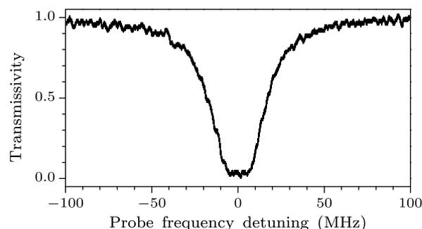
**Fig. 6.** Absorption spectrum of trapped Rb atoms in the compressed MOT, corresponding to optical density of about 16.
