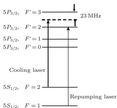
**Fig. 1.** Relevant energy diagram of the  $D_2$  line of the  $^{87}\text{Rb}$  atoms.
