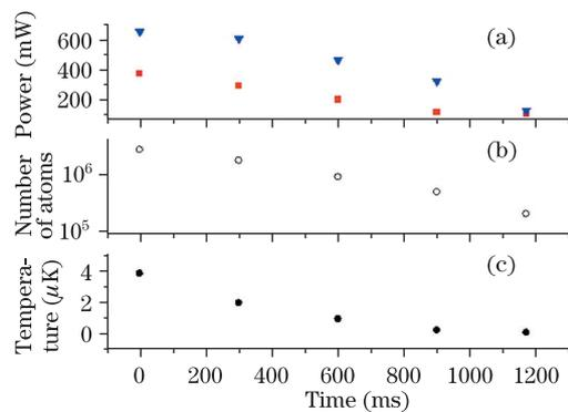
Fig. 3. Evaporation process in a crossed optical dipole trap. (a) Optical powers of two trap beams as functions of evaporation time. The squares (trigonals) correspond to the powers of the beams with the 38 (49)  $\mu\text{m}$  waist. (b) Number and (c) temperature of atoms as functions of evaporation time.
