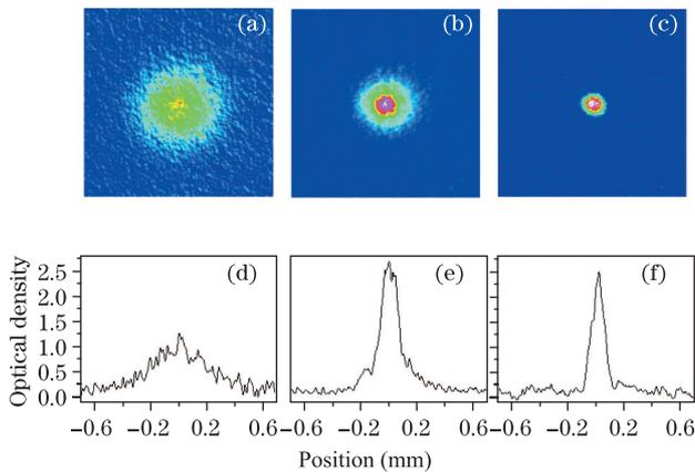
Fig. 4. Absorption images of atomic cloud and density profiles showing the appearance of BEC with 30-ms free expansion time. (a) Thermal atomic cloud of  $T=0.44 \mu\text{K}$ , which is the BEC transition point, (b) mixture of condensate and thermal cloud with  $T=0.12 \mu\text{K}$ , (c) nearly pure condensate with the number  $1.5 \times 10^5$ , and (d), (e), and (f) are the linear density profiles along the horizontal direction corresponding to (a), (b), and (c), respectively.
