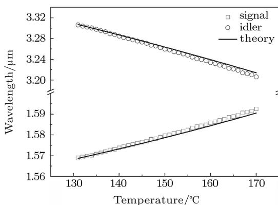
**Fig. 5.** Wavelength tuning range of the SRO as a function of PPLN temperature for a poled period of 29.8  $\mu\text{m}$ . The diamonds are the experimental results and the solid curves represent the theoretical results according to the system.
