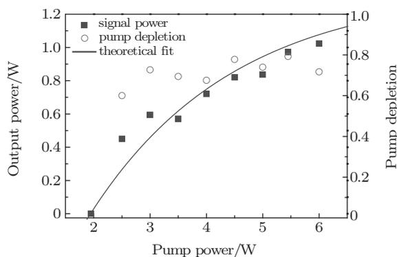
Fig. 2. Measured output power and pump depletion of SRO as a function of pump power.
