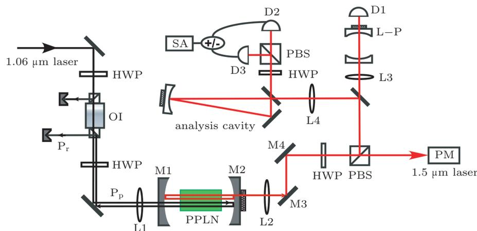
**Fig. 1.** (colour online) Experimental setup of the 1.5  $\mu\text{m}$  laser generated by an SRO. HWP: half-wave plate; OI: optical isolator; L1–L4: lens; M1–M4: mirrors; PBS: polarizing beam splitter; PM: power meter; D1–D3: detector; F–P: confocal Fabry–Perot cavity; SA: spectrum analyser; P<sub>p</sub>: pump beam; P<sub>r</sub>: reflecting pump beam.
