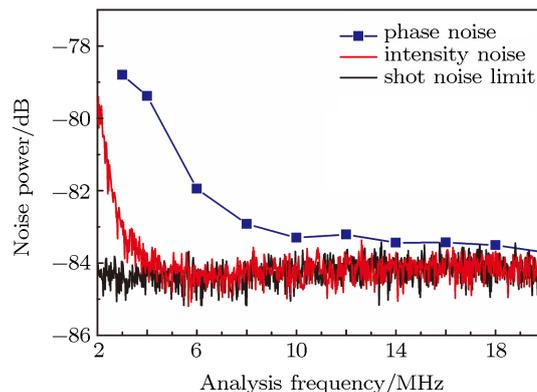
**Fig. 6.** (colour online) Measured intensity and phase noise power of 1.5- $\mu\text{m}$  laser as functions of analysis frequency. The parameters of the spectrum analyser include: the resolution bandwidth is 100 kHz, the video bandwidth is 100 Hz and the sweep time is 1.4 s.
