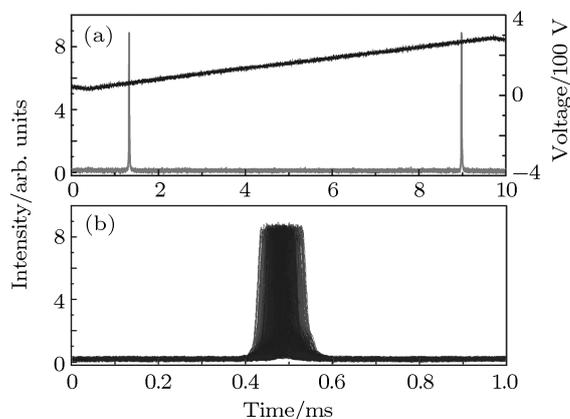
Fig. 4. Transmission intensity of the scanning Fabry-Perot interferometer.
