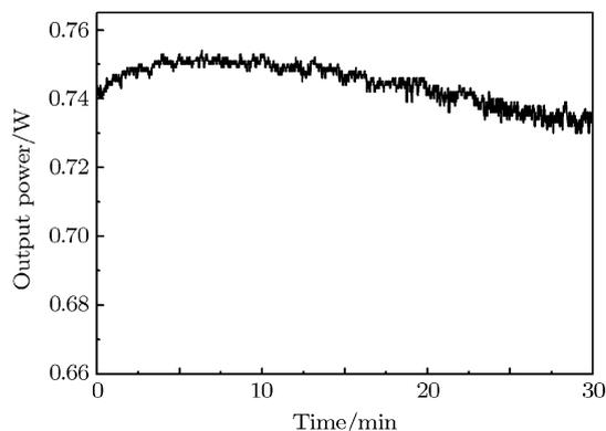
Fig. 3. Stability of the signal output at power around 0.75 W in 30 min.
