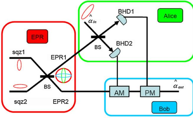
**Figure 1.** Schematic setup of the continuous-variable quantum teleportation, which consists of a source of a two-mode squeezed-vacuum state, a BS, two BHD, along with amplitude modulation and phase modulation.
