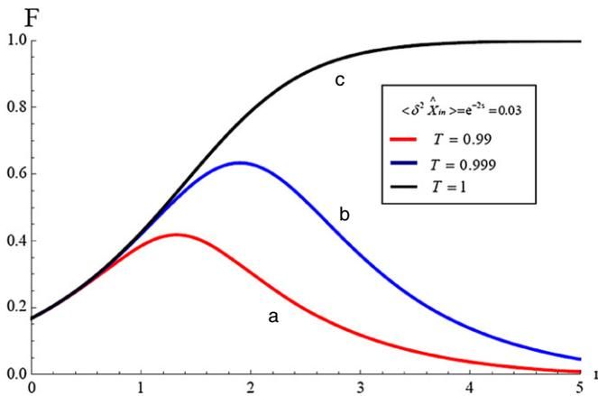
**Figure 2.** The influence of the phase-damping model on the fidelity for different EPR correlation parameters  $r$  of the noisy quantum channel. The input state with the squeezing variance  $\langle \delta^2 \hat{X}_{in} \rangle = 0.03$ . The lines  $a$ ,  $b$  and  $c$  are corresponding to the different quantum channel transmission coefficients  $T = 0.99, 0.999$  and  $1$ , respectively.
