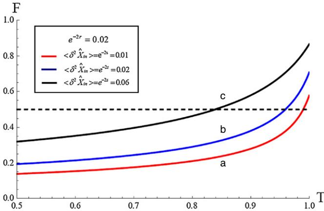
**Figure 3.** The influence of the amplitude-damping model on the fidelity, where  $r$  is the EPR correlation parameter and  $T$  is the transmission coefficient of the noisy quantum channel. The lines  $a$ ,  $b$  and  $c$  correspond to the squeezing variance of the input state  $\langle \delta^2 \hat{X}_{in} \rangle = 0.01, 0.02$  and  $0.06$ , respectively.
