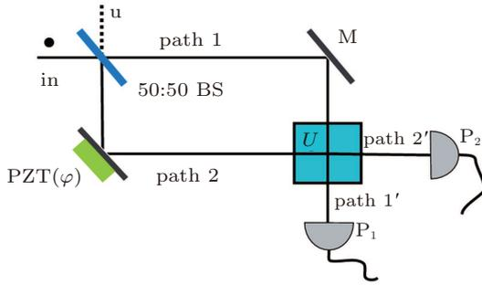
**Fig. 2.** (color online) The Mach–Zehnder interferometer setup. BS is a 50:50 beam splitter, PZT is a piezoelectric transducer, M is a mirror,  $U$  stands for an unknown device, and  $P_1$  and  $P_2$  are the single-photon detectors.
