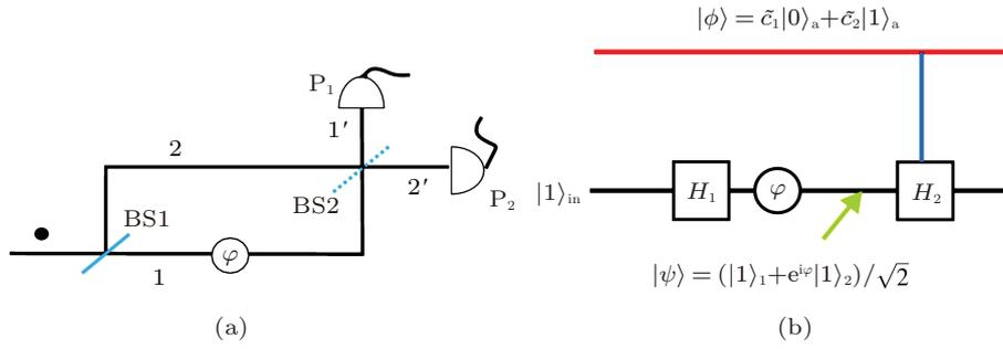
**Fig. 1.** (color online) (a) A schematic wave–particle duality experiment. By inserting or removing BS2, we can observe the wave or particle behavior, respectively. (b) Schematic diagram of a wave–particle duality experiment with a Q-BS, where the presence or absence of the second beam splitter is represented by the ancillary state  $|\phi\rangle$ , which is a superposition of its presence and absence (the second beam splitter itself is represented by a Hadamard operation  $H_2$ ).
