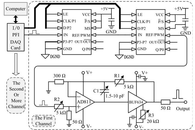
Fig. 4. Schematic diagram of the pulse generator.
