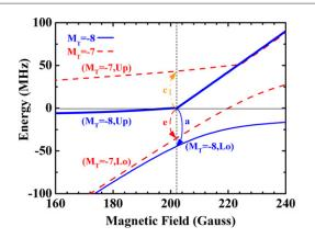
**Figure 1.** Energy spectrum of relevant molecular levels of  $^{40}$ K $_2$  versus the magnetic field in the electronic ground state. The zero of energy is taken to be that of two separated atoms  $|9/2, -9/2\rangle + |9/2, -7/2\rangle$  at each magnetic field strength.  $M_T$  is total angular momentum projection  $M_{F_1} + M_{F_2}$
