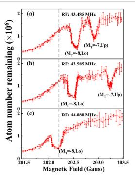
**Figure 3.** Atom loss from the entrance channel  $|9/2, -9/2\rangle$ ,  $|9/2, -7/2\rangle$  in the vicinity of the Feshbach resonance 202.2 G for different frequencies of the RF field. (a) The frequency of the RF field is 43.485 MHz. (b) 43.585 MHz. (c) 44.080 MHz.
