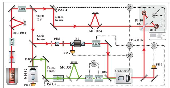
**Fig. 1.** Schematic of the experimental setup. MC, mode cleaner; PBS, polarization beam splitter; FI, faraday isolator; EOM, electro-optical modulator; OPA, optical parametric amplifier; OPO, optical parametric oscillator; DBS, dichroic beam splitter; SHG, second harmonic generation; EOAM, electro-optic amplitude modulator; PZT, piezoelectric transducer; PD, photodetector; BHD, balanced homodyne detection.
